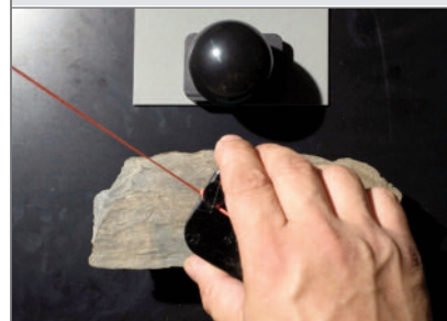
FIGURE 4. Highlight on a reflective sphere placed in the scene of an image sequence. The person holding the string is measuring the distance for the light during set up.
