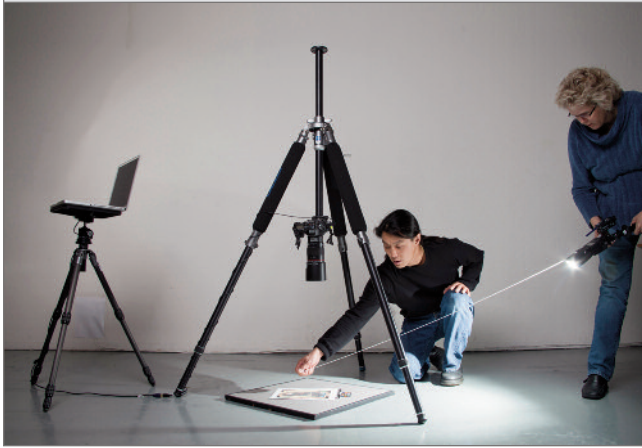
FIGURE 3. A typical highlight RTI setup with camera facing down to shoot an object on the floor. The camera is connected to a laptop computer. A radio trigger on the camera fires the flash when the camera is triggered. A string is used to keep an equal distance for the light from each position.
